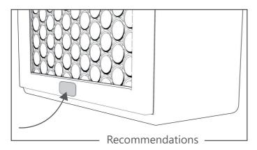
In case of use with the Ultimaker Air Manager system, we recommend using the sticker to ensure filter detection.
