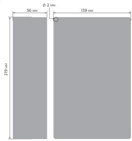
Dimensions include the sealing foam ± 0.5mm.
